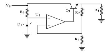
The breakdown voltage of the Zener is 5 V.  $\beta$  for the transistor is 100.  $R_1=10~k\Omega$ ,  $R_2=90~k\Omega$ ,  $R_3=30~k\Omega$ ,  $R_4=50~k\Omega$ . Calculate the total output voltage.
