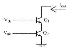
Given that  $g_{m_1}=30~\text{m}\,\Omega^{-1}$  and  $g_{m_2}=50~\text{m}~\Omega^{-1},~\alpha_1=1.1,~\alpha_2=1.5$ . What is the transconductance of the entire network ?
