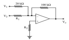
If  $V_1 = 0.2 V$ ,  $V_2 = 0.6 V$  and V0 = -7, and the op-amp is ideal, the value of  $R_1$ is :
